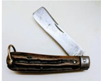
Square-point rope knife . Used by the Royal Navy and the merchant marine, and also supplied to the British military – see section 5.1 here .
