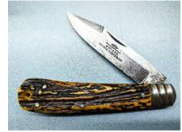
Clip-point sailor knife – more commonly found with a closed length of 4 inches, with the one shown above having a closed length of 5 inches – see section 5.3 here .
