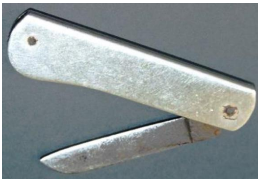
3. Rarer examples have stainless steel bodies as shown in this example. Note the larger style sheep foot blade.
