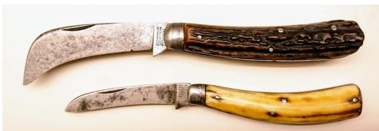
Photo 2. Top: Johnson Western Works, length closed 4 5/8 inches closed. Stag scales. hawkbill blade. Bottom: John Petty and Sons, length 4 1/8 inches closed, smooth bone scales, 'hooked pruner' blade - probably peach pruner. SOURCE: author's collection
