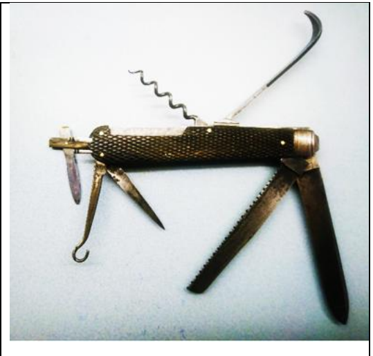
Maker: not known. All blades stamped "ARMY & NAVY C.S.L." Length closed 6 ¾ inches. Scales are Checkered Horn.
